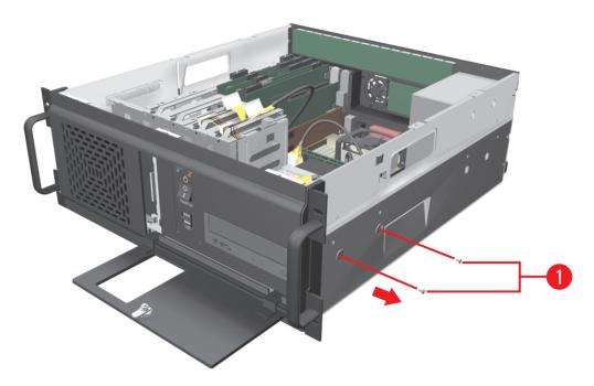
Figure 9. Removing CD/DVD Mounting Screws
